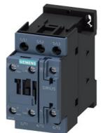
power contactor, AC-3e/AC-3, 32 A, 15 kW / 400 V, 3-pole, 42 V AC, 50/60 Hz, auxiliary contacts: 1 NO + 1 NC, screw terminal, size: S0, upright mounting position
