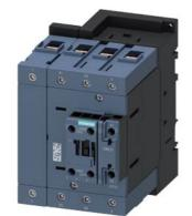
power contactor, AC-3, 65 A, 30 kW / 400 V, 4-pole, 175-280 V AC/DC, 50/60 Hz, with integrated varistor, main contacts: 2 NO + 2 NC, auxiliary contacts: 1 NO + 1 NC, screw terminal, size: S3
